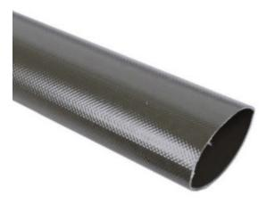
Oilvey 10 is one type of through-the-weave polyurethane (PU) covered hose. Oilvey 10 hoses shall be made from 100% high tenacity synthetic yarn circular woven and completely, totally embedded in the PU compound, excellent protected against mechanical damage, forming a single homogenous construction without the use of any glues or adhesives of any type.
