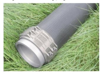
Longman 600 is one type of through-the-weave Nitrile Rubber (NBR) covered hose. Longman 600 hoses shall be made from 100% high tenacity synthetic yarn circular woven and completely, totally embedded in the NBR/PVC compound, excellent protected against mechanical damage, forming a single homogenous construction without the use of any glues or adhesives of any type. NBR compound is composed of NBR and PVC. High percentage of NBR content contributes to better abrasion-resistance.
