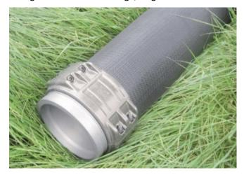
Longman 600 is one type of through-the-weave Nitrile Rubber (NBR) covered hose. Longman 600 hoses shall be made from 100% high tenacity synthetic yarn circular woven and completely, totally embedded in the NBR/PVC compound, excellent protected against mechanical damage, forming a single homogenous construction without the use of any glues or adhesives of any type. NBR compound is composed of NBR and PVC. High percentage of NBR content contributes to better abrasion-resistance.
