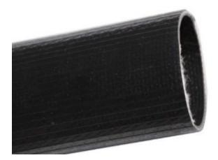
Longman 450 is one type of through-the-weave Nitrile Rubber (NBR) covered hoses. Longman 450 hoses shall be made from 100% high tenacity synthetic yarn circular woven and completely, totally embedded in the NBR/PVC compound, excellent protected against mechanical damage, forming a single homogenous construction without the use of any glues or adhesives of any type. NBR compound is composed of NBR and PVC. High percentage of NBR content contributes to better abrasion-resistance.
