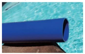
Potaflow is one type of through-the-weave polyurethane (PU) covered hose which is made of PU materials approved according to NSF 61 standard. Potaflow hoses shall be made from 100% high tenacity virgin synthetic yarn circular woven and completely, totally embedded in the PU compound, excellent protected against mechanical damage, forming a single homogenous construction without the use of any glues or adhesives of any type.
