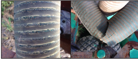
PVC Hose cracking due to UV exposure
